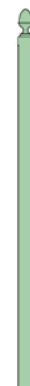
FULL POST END POST FIELD POST CORNER POST W:4" D:4" H:82" or UNDER- GROUND H:96"
